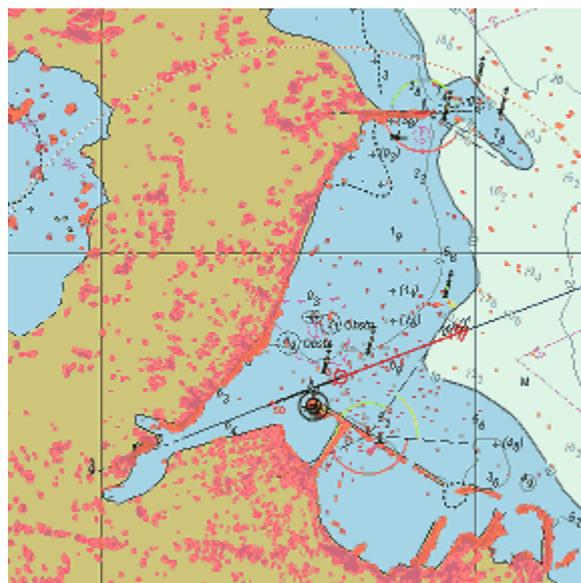
The **Radar Navigation Module (RNM)** has been designed for solving of a wide range of navigational tasks. Together with the dKart Navigator electronic chart systems **RNM** provides means for displaying of a full radar image atop of an electronic chart. The possibility of simultaneous/separated monitoring of the ENC and radar image let a navigator take
