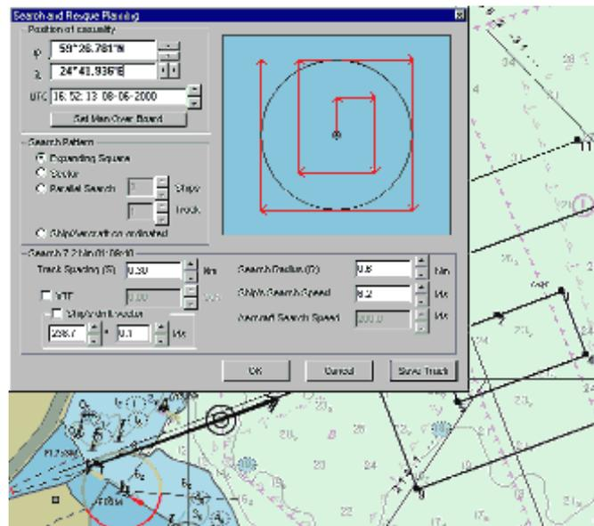
This module provides all the necessary means for planning, monitoring and information support of Search and Rescue operations in full accordance with IMO MERSAR and IMOSAR recommendations. It is possible to plan one-ship, multiple-ship, ship/aircraft S&R operations in different modes basing on the ship's drift vector, visibility distance, Man over Board sensor data and so on.
