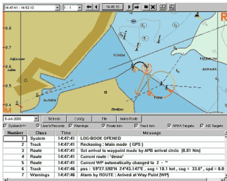
The principal navigational information that includes ship movement and radar targets data, an information on changes in operation mode of the navigational system and onboard devices, ship's motion settings, navigator's own narration, etc are being logged automatically in an electronic navigational logbook.
