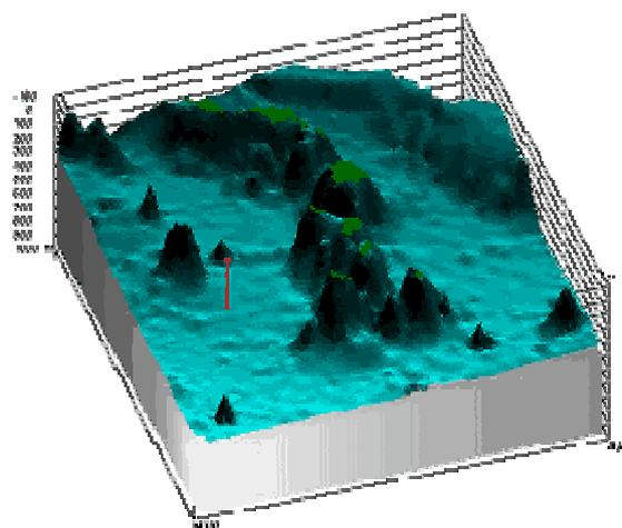
This function allows creation and viewing of 3-dimensional model of the sea bottom. As a source of information an ENC data and echosounder information are used. The possible applications of this function are: maneuvering in narrow waters and unfamiliar navigation areas; hydrographic activities, fishing, etc.
