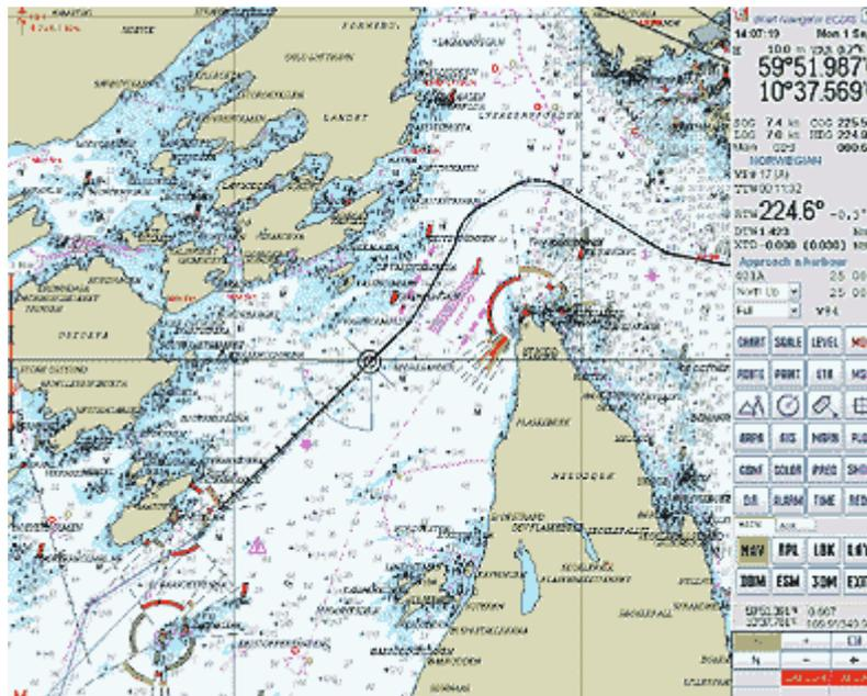
**dKart Navigator** is an electronic navigation chart system specially designed to facilitate all the navigational tasks of mariner's day-to-day practice. Along with displaying vector nautical charts (both S-57 official data and CM93 world coverage) it offers:
